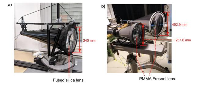
**Figure 1:** Lens-based radioluminescence detection setups developed at the PTB (M. Luchkov, V. Dagendorf, F. Krasniqi). (a) Fused-silica lens (Abet Technologies) system mounted on a goniometer and rotation stage (Newport M-BGM160PE and RVS80CC). (b) PMMA Fresnel lens (Orafol Fresnel Optics) systems. All lens systems can be coupled to selected PMTs and UV-C or UV-A interference filters.
